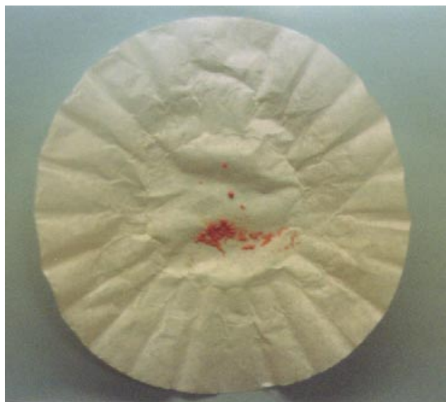
Figure 9. Isolation of color-changing component from orange Silly Putty using a coffee filter.
