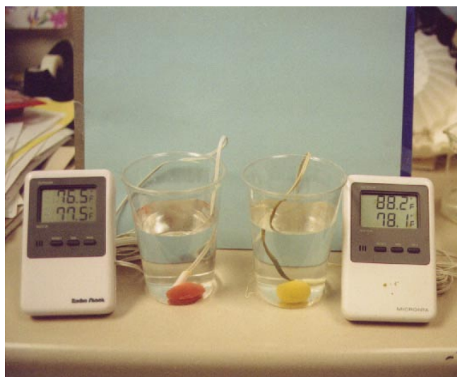
Figure 10. Determining the temperature range of the color change for orange Changeable Silly Putty.
